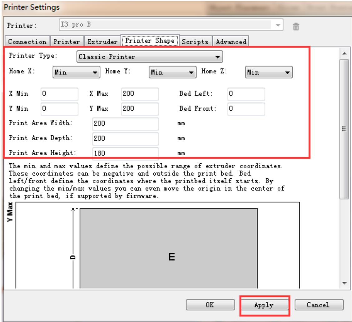
If the object which is being printed is not in the center of the hot bed, you can adjust the following two values to compensate for the distance deviation of X / Y direction:
