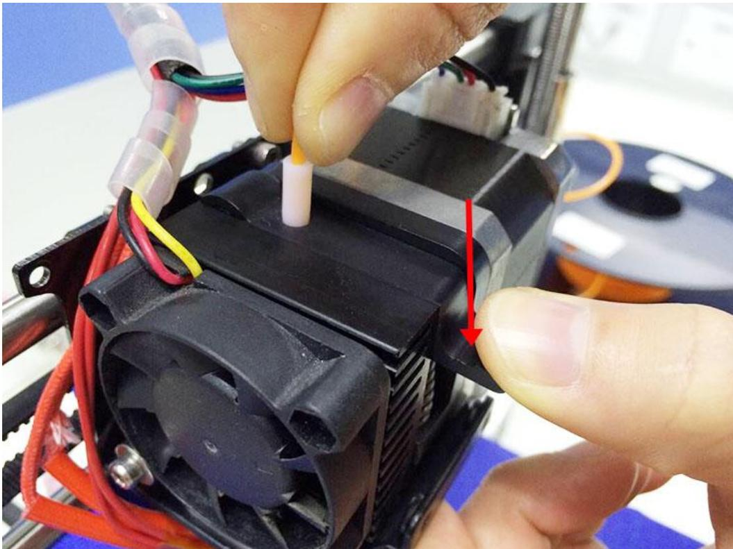
After pushing the filament into the bottom of hotend, use the feeding button on Repetier (as shown in following picture) to do manual feeding. If the nozzle can extrude filament fluently, the extruder
