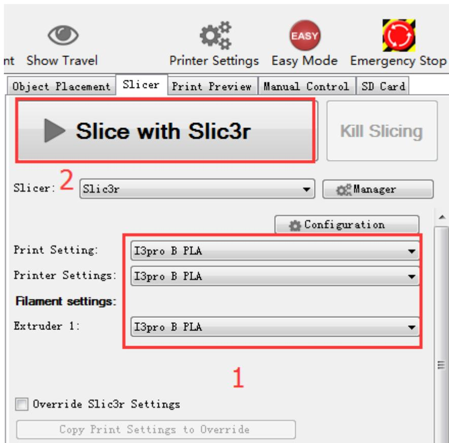
In this way, .gcode file which can be recognized by the printer is generated.
